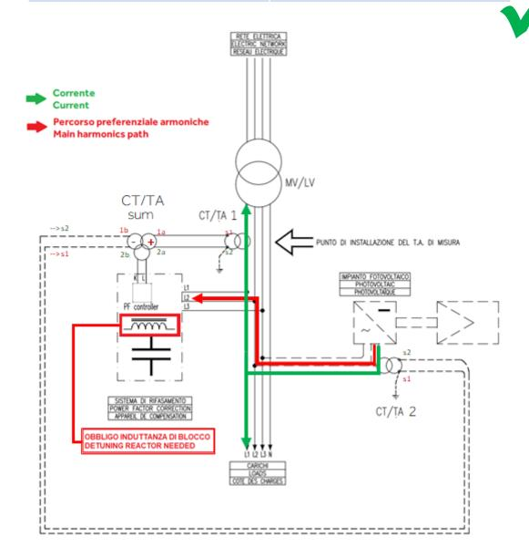
When an optimal solution (see 'CASE 1') is not possible, the above 'escamotage' may be used to have the APFC more effective:
