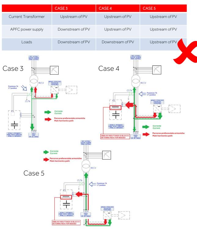
The current drawn by the Loads crosses the CT to a lesser extent because the PV supplies all or part of the ACTIVE power to the users (depending on the difference between the PV power and the power required by the Loads), reducing the current flowing through the CT to only the REACTIVE fraction.
