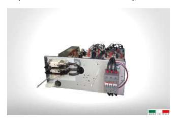
The RCL series drawers are designed for our G9E-type cabinets. Inside each drawer are assembled triads of single-phase capacitors. The versions shown in the catalogue are all equipped with blocking inductors, for applications with a high level of current harmonic distortion.
