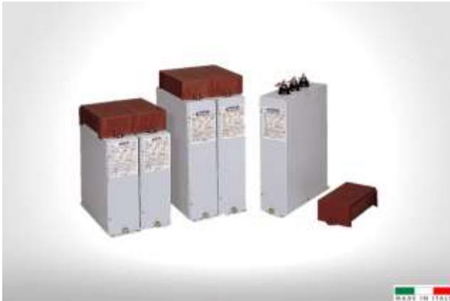
The three-phase modular capacitors of the **CT** series are designed for fixed low-voltage power factor correction. The construction of the capacitors is designed to guarantee optimum thermal dissipation. Three single-phase MKAS units are assembled inside, each equipped with an anti-explosion device.
