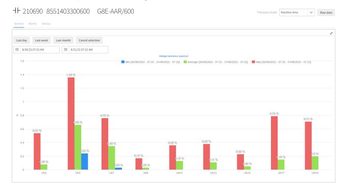
The **Harmonic Spectrum in Current** is shown below when the photovoltaic generates almost all of the current absorbed by the load:
