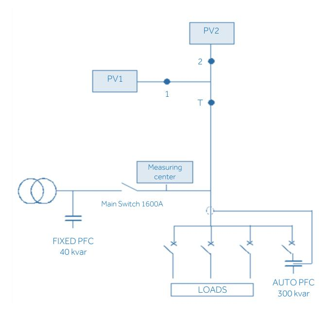
In this case the capacitor bank is an  $\underline{AAR/600}$ , of 300kvar with steps of 25 + 50 + 3x75 kvar, for THD (I) max. = 100% and THD (U) max. = 6% in the network.
