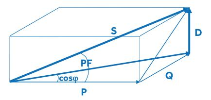
In the case of distorting power, sometimes machinery malfunctions are also generated, such as the blocking of correct PLC operation or even breakage of electronic devices (eg controlled diodes, IGBTs, electronic boards...). <u>The distorting power is essentially due to the harmonic currents generated by electronic systems</u>, particularly heavy is harmonic pollution due to the third harmonic (generated by single-phase electronic systems such as LED lighting and computers).
