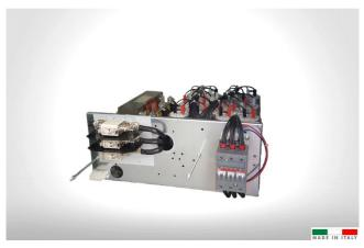
The RCL series racks are designed for our G9E type cabinets. Inside each rack are assembled single-phase capacitor terns. The versions shown in the catalog are all equipped with blocking rectors, for applications with a high level of harmonic current distortion.
