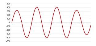
Among the main causes of the jolts are the sudden shutdown of large loads and the anomalous switching of the power factor correction capacitors.
