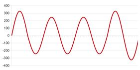
Among the most common symptoms of sags are dimming of incandescent lights, computer lockups, shutdowns of sensitive electronic equipment, loss of data (memory) of programmable controllers and problems in relay control. In these cases, it is advisable to start by monitoring the load so that the symptoms of the drop occur first. If there is no correlation, move further upstream, until you can trace the origin.
