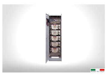
FAM05/07 is realized by appropriately tuning in frequency, a battery of capacitors and a three-phase reactance. In this way a resonant circuit is realized which is chosen as the preferred way from the harmonic current which is to be reduced, and is equipped with a  ${\bf microprocessor}$   ${\bf control}$   ${\bf system}$  for inserting modules. Features:
