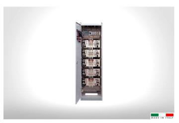
**FAM05** is realized by appropriately tuning in frequency, a battery of capacitors and a three-phase reactance. In this way a resonant circuit is realized which is chosen as the preferred way from the harmonic current which is to be reduced, and is equipped with a **microprocessor control system** for inserting modules. Features:
