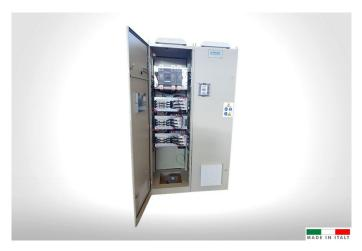
The entire **B35-ST** series is equipped with "zero-crossing" static relays (thyristors), and it has been designed to improve the performance of traditional equipment, such as: increasing the life of the capacitors banks, decreasing the time response of the equipment to follow rapid changes in loads with a **medium-low harmonic distortion**.
