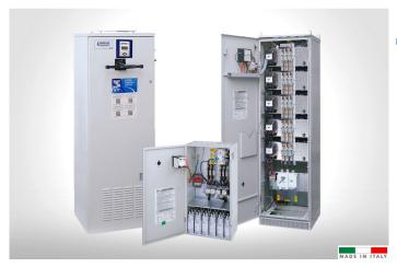
**B15** series equipment are particularly suitable for three-phase networks with operating voltage equal to 400 Vac (+/- 10%) with low harmonic distortion in current. These equipment quarantee an accurate P.F.C., thanks to a multi-step design that effectively divides the power. In addition, on the G6E and G8E cabinet, all the capacitors banks are assembled on racks, easily removable from the front of the panel, for simple management and maintenance.
