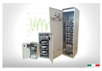
**B15** series equipment are particularly suitable for three-phase networks with operating voltage equal to 400 Vac (+/- 10%) with low harmonic distortion in current. These equipment quarantee an accurate P.F.C., thanks to a multi-step design that effectively divides the power. In addition, on the G6E and G8E cabinet, all the capacitors banks are assembled on racks, easily removable from the front of the panel, for simple management and maintenance.
