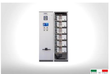
AAR/600 series equipment are particularly suitable for threephase networks with high harmonic distortion in current. These equipment guarantee an accurate P.F.C., thanks to a multi-step design that effectively divides the power. In addition, on the G6E and G8E cabinet, all the capacitors banks are assembled on racks, easily removable from the front of the panel, for simple management and maintenance.
