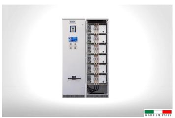
AAR/600 series equipment are particularly suitable for threephase networks with high harmonic distortion in current. These equipment quarantee an accurate P.F.C., thanks to a multi-step design that effectively divides the power. In addition, on the G6E and G8E cabinet, all the capacitors banks are assembled on racks, easily removable from the front of the panel, for simple management and maintenance.
