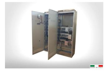
The entire **AAR/100-ST** series is equipped with "zero-crossing" static relays (thyristors), and it has been designed to improve the performance of traditional equipment, such as: increasing the life of the capacitors banks, decreasing the time response of the equipment to follow rapid changes in loads. Suitable for applications with high harmonic distortion such as automotive, harbours, mechanical workshops, ...
