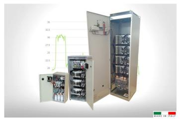
**B50** series equipment are particularly suitable for three-phase networks with operating voltage equal to **400 Vac** (+/- 10%) with **medium harmonic distortion** in current. These equipment guarantee an accurate P.F.C., thanks to a multi-step design that effectively divides the power. In addition, on the G6E and G8E cabinet, all the capacitors banks are assembled on racks, easily removable from the front of the panel, for simple management and maintenance.
