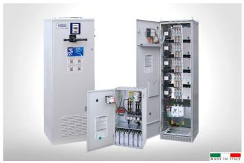
B35 series equipment are particularly suitable for three-phase networks with operating voltage equal to 400 Vac (+/- 10%) with low-medium harmonic distortion in current. These equipment guarantee an accurate P.F.C., thanks to a multi-step design that effectively divides the power. In addition, on the G6E and G8E cabinet, all the capacitors banks are assembled on racks, easily removable from the front of the panel, for simple management and maintenance.
