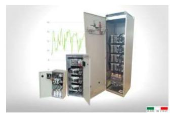
**B15** series equipment are particularly suitable for three-phase networks with operating voltage equal to **400 Vac** (+/- 10%) with **low harmonic distortion** in current. These equipment guarantee an accurate P.F.C., thanks to a multi-step design that effectively divides the power. In addition, on the G6E and G8E cabinet, all the capacitors banks are assembled on racks, easily removable from the front of the panel, for simple management and maintenance.
